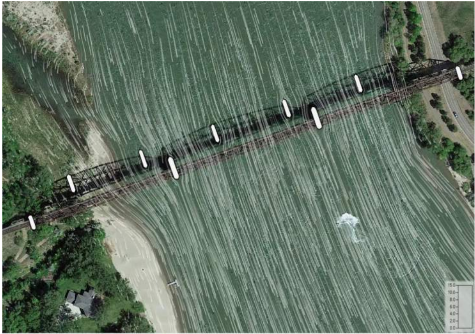
Existing Bridge and New Bridge 42.5-feet Upstream - Two-Dimensional Modeling
